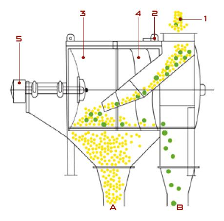
Working principle of Drum Sieve Machine
