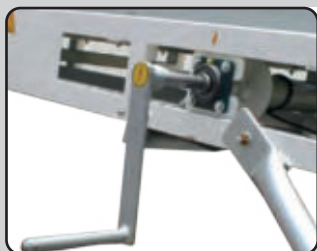
Jack Lift : Inclination height adjusted with Manually Controlled Jack Lift.
