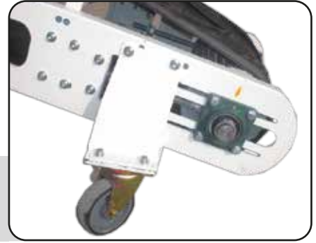
Tail end equipped with two small wheels for maneuvering.
