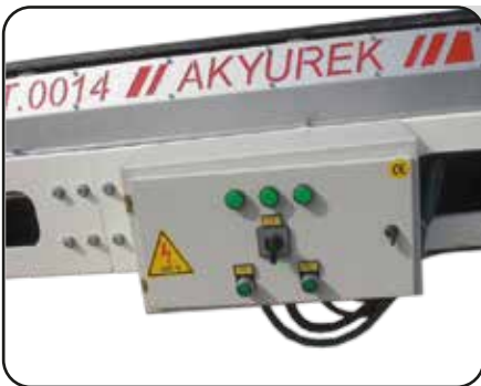
On Board Power Panel
