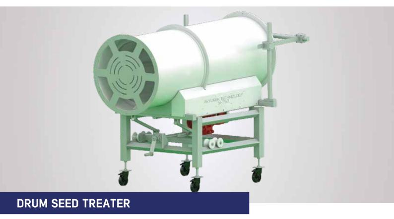
The DST Basic series treater is designed to continuously apply single or multiple products, simultaneously, to predefined quantities of seed, which is established through calibration.
